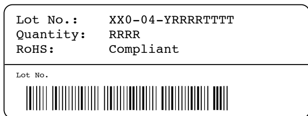
Figure 19: First label on reel: XX = Sensor Type (11 for SHT11), 04 = Chip Version (V4), Y = last digit of year, RRRR = number of sensors on reel, TTTT = Traceability Code.
